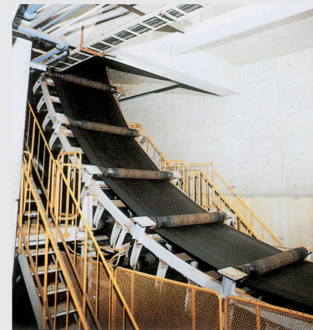
③ 下部曲率部 (R部) Low side curved section ("R" section)
